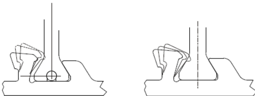
Figure 2 – Example of strip installation
